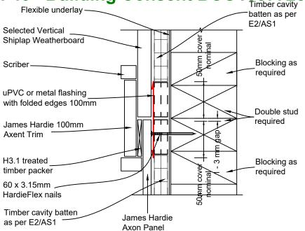
**VERTICAL JUNCTION BETWEEN** VERTICAL SHIPLAP WEATHERBOARD AND JAMES HARDIE AXON PANEL
