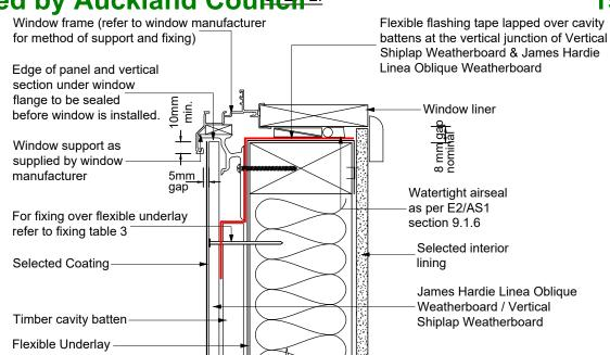
WINDOW SILL DETAIL - AT THE VERTICAL JUNCTION OF VERTICAL SHIPLAP WEATHERBOARD & JAMES HARDIE LINEA OBLIQUE WEATHERBOARD
