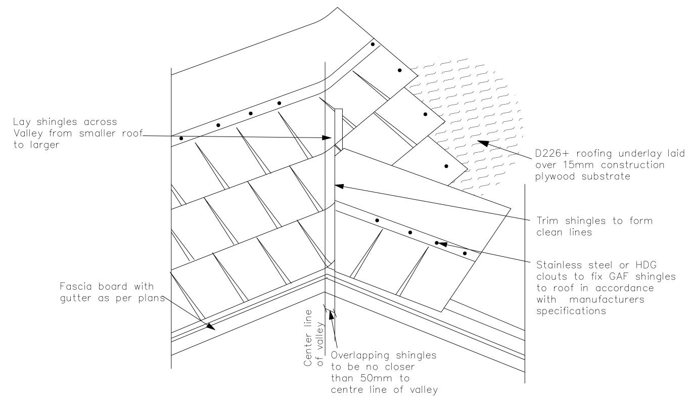
GAF Asphalt Shingles Detail - Valley cladding (NTS)
