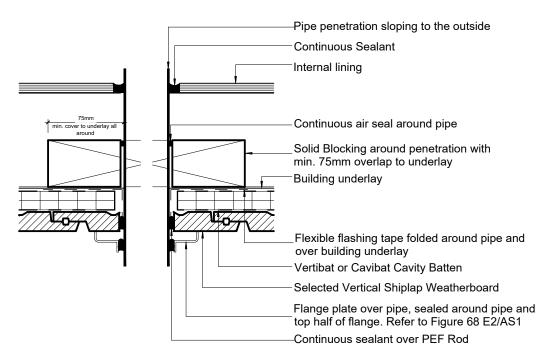
Vertical Shiplap Weatherboard - Pipe Penetration (Plan View)
