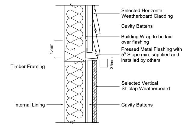
Horizontal Weatherboard & Vertical Shiplap Weatherboard - Horizontal Junction Detail
