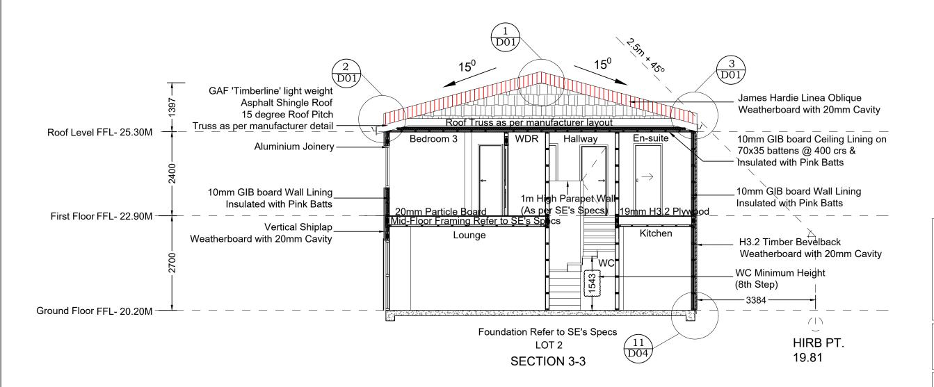
Make sure a minimum 25mm air gap will be maintained between the top of the insulation and the underside of the roofing underlay. Refer BRANZ house Guideline & NZBC E3/AS1 clause 1.1.3
