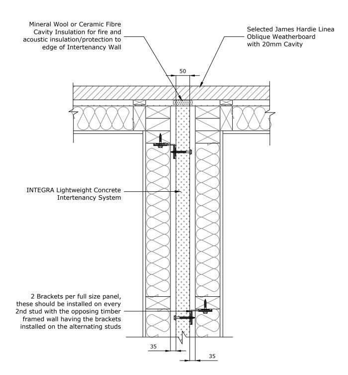
DETAIL AT EXTERNAL TIMBER FRAME WALL (PLAN VIEW) - WEATHERBOARD
