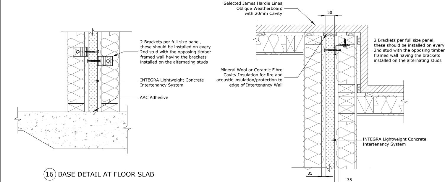
(17) DETAIL AT EXTERNAL TIMBER FRAME WALL (PLAN VIEW) - LINEA WEATHERBOARD
