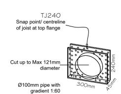
PIPE THROUGH JOIST DETAIL
