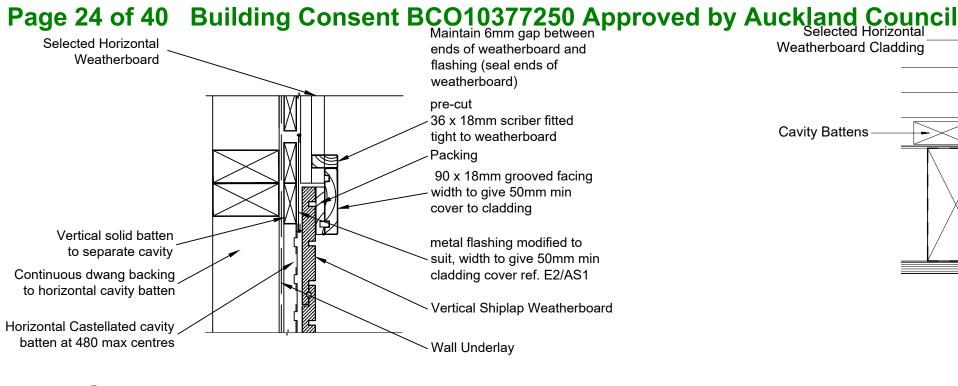
Horizontal Weatherbaord & Vertical Shiplap Weatherboard - Vertical Junction Detail
