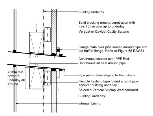
Vertical Shiplap Weatherboard - Pipe Penetration Detail
