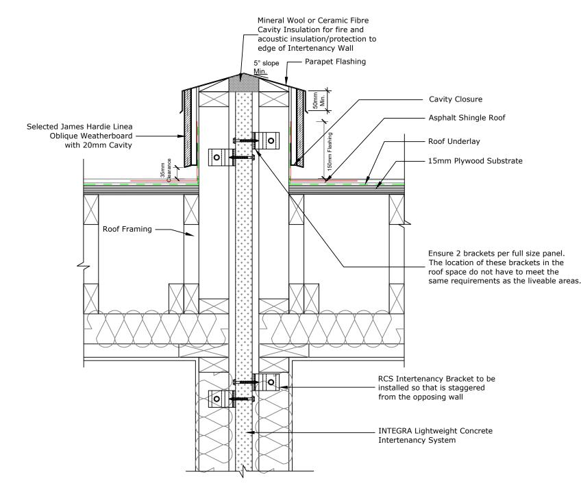
DETAIL AT ROOF / CEILING (END ELEVATION)
