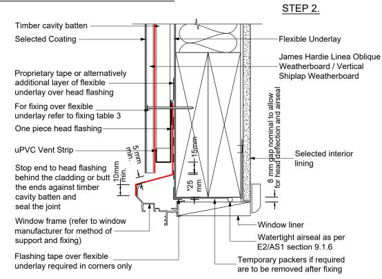
WINDOW HEAD DETAIL - AT THE VERTICAL JUNCTION OF VERTICAL SHIPLAP WEATHERBOARD & JAMES HARDIE LINEA OBLIQUE WEATHERBOARD
