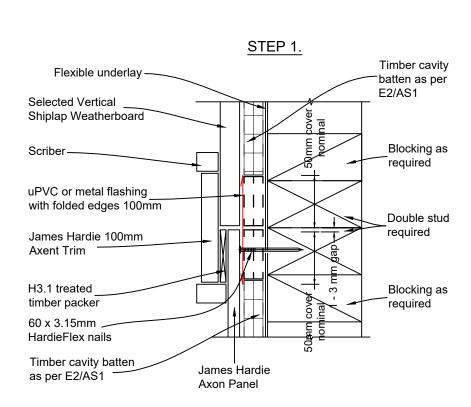
**VERTICAL JUNCTION BETWEEN** VERTICAL SHIPLAP WEATHERBOARD AND JAMES HARDIE AXON PANEL
