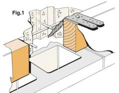
1. Bottom Plate Fixing Anchors shall be fixed at 900mm centres max. to the boxing for concrete floor slabs, over a continuous vapour barrier. Each Fixing Anchor is nailed prior to concrete pour, and shall be left undisturbed until concrete has hardened
